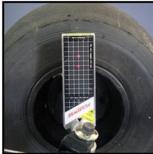
Now fit the wheels on your kart with the units still on and place it on a flat, level surface. Place the driver in the kart, this is the 'dynamic' setting as it shows you what your alignment will look like while on the track.
