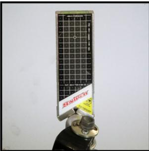
Make sure the Spindles and Magnetic Vee Block are clean and free of debris before attaching the Snipers. Fit your Snipers by carefully placing them onto the spindles with the forward arrows facing the front of the kart. These units will fit any diameter up to 63mm (2 1/2 inch), for non magnetic spindles simply use a cable tie or similar to attach the units.
